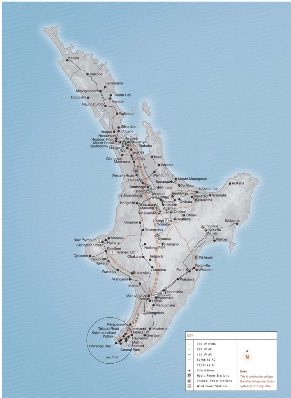
Figure 87 - North Island power system
