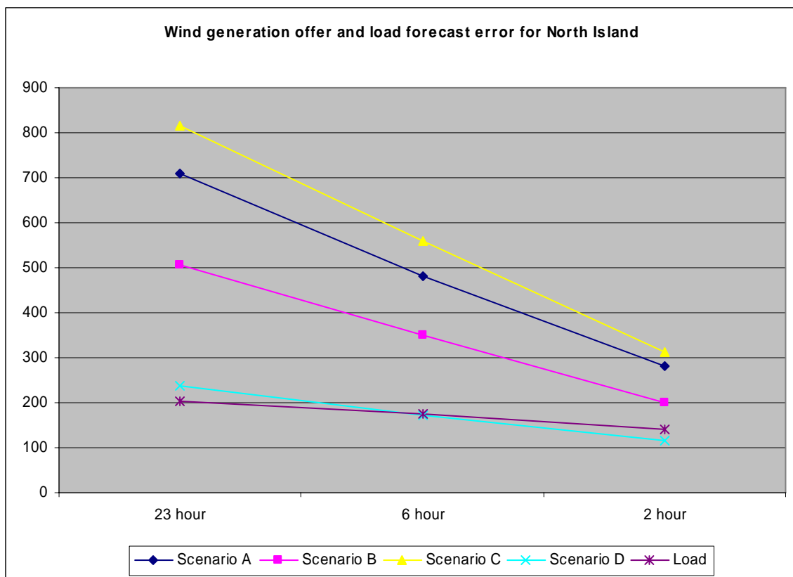
Figure 8: Wind generation forecast and SO load forecast errors for the North Island expected to occur once per day (based on Garrad Hassan [2])
